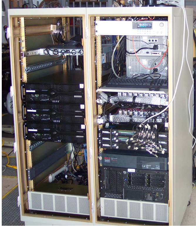
Figure B.5: The double-wide data acquisition rack contains both the 40-channel system and old 20-channel system for backup purposes. It was located in the data acquisition room in the Gregorian dome. Parts of the 40-channel system were removed to continue software development.
