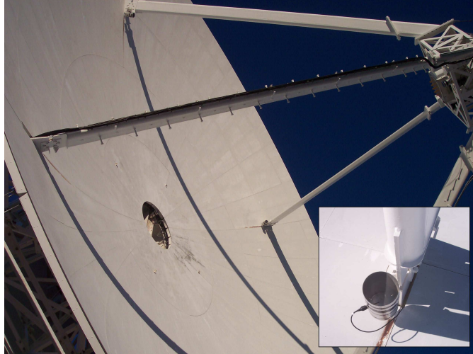
Figure 3.12: Calibration horns mounted on the Green Bank 20-Meter Telescope. Inset is a closer look at one of the horns attached to a feed arm.
