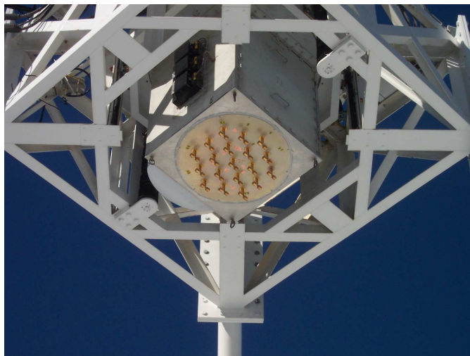
Figure 3.9: The BYU active-impedance-matched 19-element Carter PAF: hexagonally spaced half-wave thickened dipoles, separated by 0.6\lambda on a ground plane. The PAF is attached to the end of the front-end box which is mounted to the 20-Meter Telescope. The front end box contains the LNAs, receiver cards, power supplies, and LO distribution hardware.
