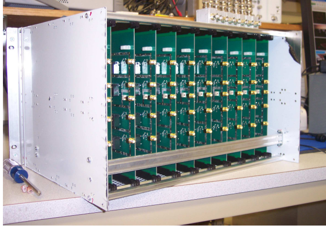
Figure B.3: Rack mount card cage holding the receiver cards. The ten receiver cards were installed on rails so that they could easily slide in and out of position. Ample room was provided to install cables on both the front and back side.
