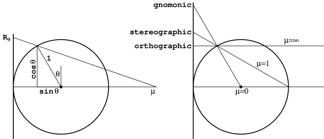
Fig. 4. (Left) geometry of the perspective zenithal projections: (right) the three important special cases.
