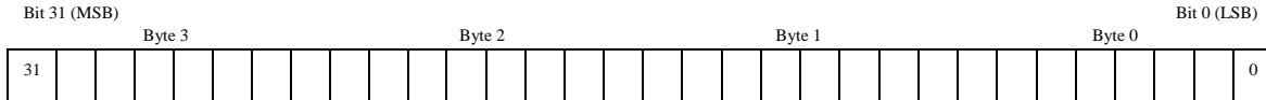
Figure 4: Real 1-bit/sample data-word format (numbers in boxes indicate relative sample #'s in time order); byte #'s indicate relative byte address within 32-bit word (little endian format).
