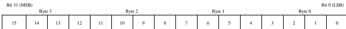
Figure 16: Data Array word for complete-sample length of 2 bits (i.e. 2^n * 2^k = 2 ); relative sample times are indicated in each 2-bit complete sample; byte #s indicate relative byte address within 32-bit word (little endian format)
