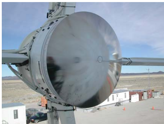
Figure 2. Evaluation Receiver Installed. Figure 3. Nutating Subreflector Installed
